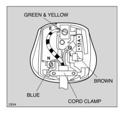
The plug moulded onto the lead incorporates a 13amp BSI362 fuse. Only ASTA or BSI fuses should be used.
